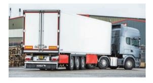
importantly, where lifting axles aren't fitted, our EBS can dump air out of the rear axle suspension, which again reduces the turning circle and saves on scrub."
